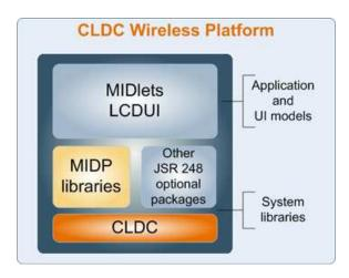
FIGURE 4-1 CLDC WIRELESS PLATFORM<sup>11</sup>
