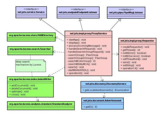
FIGURE 4-8 JXME PROXY CLASS DIAGRAM
