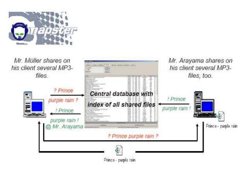
FIGURE 2-6 NAPSTER ARCHITECTURE [WEHR06]
