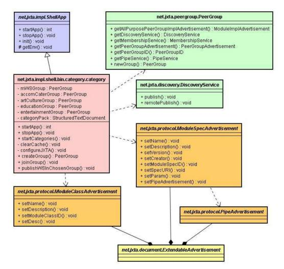
FIGURE 4-4 SERVICE PROVIDER CLASS DIAGRAM
