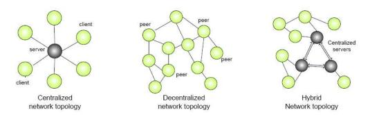
FIGURE 2-5 DIFFERENT NETWORK TOPOLOGIES
