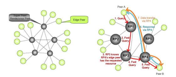
FIGURE 2-8 MIXED P2P AND OPERATING PRINCIPLE OF JXTA [HYAR04]
