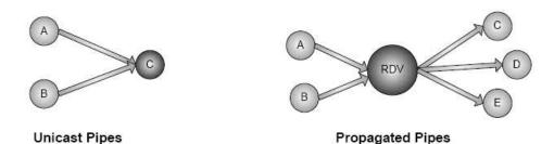
FIGURE 2-10 JXTA PIPES [JXTA07]
