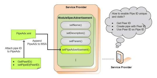
FIGURE 4-5 TO ATTATCH A PIPE AD TO MSA
