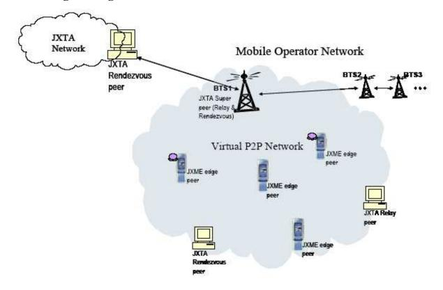
Figure 22 : General Architecture of Mobile Hosts in JXTA network [43].
