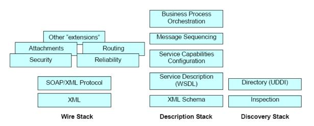
Figure 15 : Web Services Conceptual Architecture (by IBM) [16].
