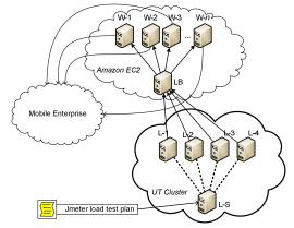
Figure 2. Load test setup for the MWSMF
