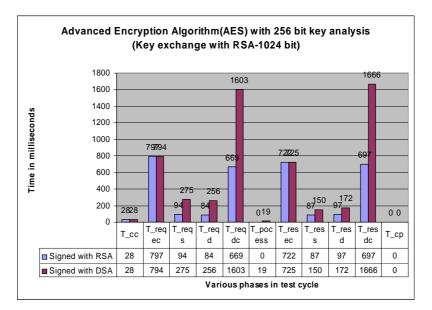
Fig. 14. Latencies of various phases of a message-level secured mobile web service invocation cycle.
