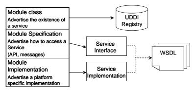
Fig. 18. Mapping between JXTA modules and Web Services.
