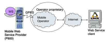
Fig. 4. The operational setup of Mobile Host in a live GPRS environment.
