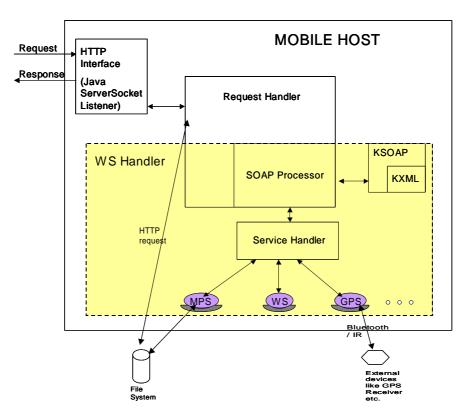
Fig. 2. Core architecture of the Mobile Host
