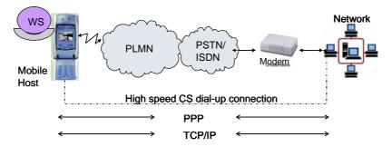
Fig. 3. Architecture for an end-to-end TCP/IP connection between the mobile terminal and the prototyping network using HSCSD connection.
