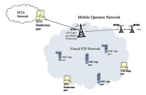
Fig. 17. Virtual mobile P2P network with Mobile Hosts.
