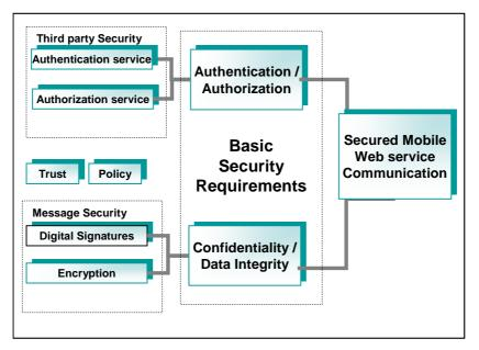
Fig. 8. Basic security requirements for mobile web services.
