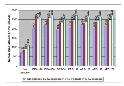
Fig. 13. Performance latencies with various symmetric key encryption algorithms and exchanging keys with RSA 1024.
