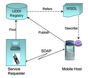
Fig. 1. Basic mobile web services framework with the Mobile Host.
