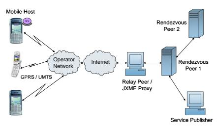
Fig. 20. The P2P based mobile web service discovery evaluation scenario.
