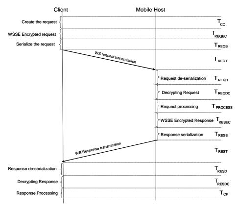
Fig. 12. Secured mobile web service invocation: operations and time stamps.
