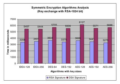
Fig. 15. Comparison of timestamps of web service invocation cycle with various symmetric key encryption algorithms.
