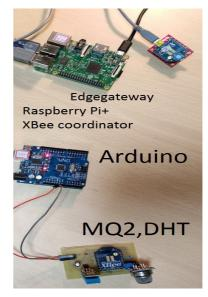
Fig.7 Edge gateway connected with different sensors
