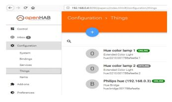
Fig. 2 An instance of an openHAB configuration panel
