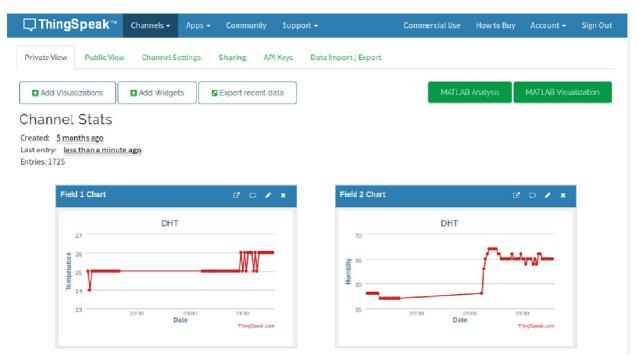
Fig.8 ThingSpeak cloud visualization of sensor data
