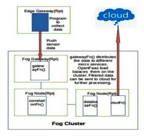
Fig.5 Distributed deviceless Platform
