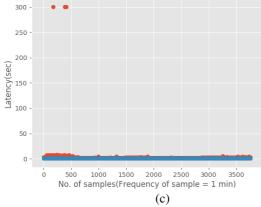
Fig.9 a) DHT11 sensor data latency comparison between cloud and fog nodeb) MQ135 sensor data latency comparison between cloud and fog nodec) MQ2 sensor data latency comparison between cloud and fog node
