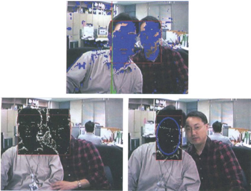
Figure 11.10. Occlusion between two faces (top); Sobel edge within the ROI (bottom-left); ellipse fitting (bottom-right).
