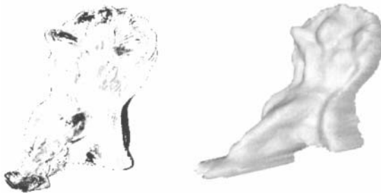
Figure 9.14. Left: Difference (scaled) between the two disparity maps in Fig. 9.14. Right: Shaded representation of the scene "Tom" reconstructed with projected color code (reprinted from [Kle et al. 96] with permission from Vieweg).
