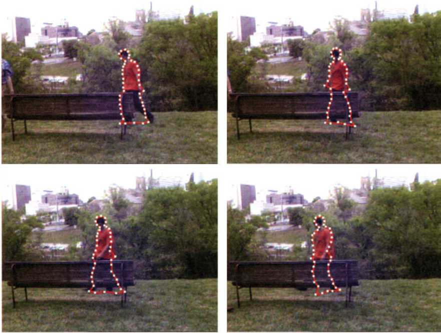
Figure 11.22. Fitting results in four frames of a video sequence with a partially occluded person. The hierarchical method with the median selection mode in the RGB color space was used (reprinted from [Kos et al. 03] with permission from Elsevier).
