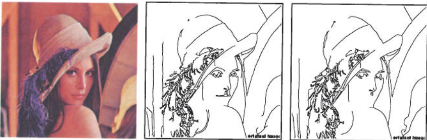
Figure 6.3. Results of edge detection applied to the color image "Lena" (left) for a color variant of the Canny operator (center) and the gray-level algorithm of the Canny operator (right) (with friendly permission from John Owens, Stanford University).
