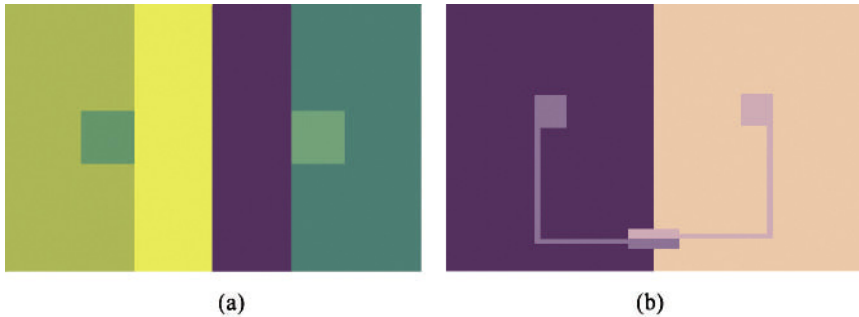
Figure 13.2. Simultaneous contrast can make (a) the same colors look different, or (b) different colors look the same [Tay86].
