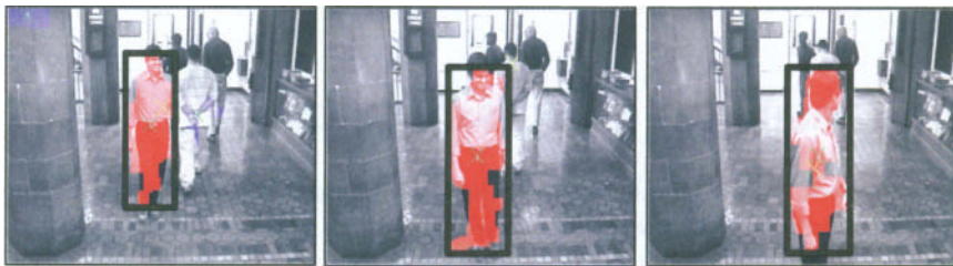
Figure 11.5. Sequence of frames from the PTZ camera showing achieved handover (successive target views).
