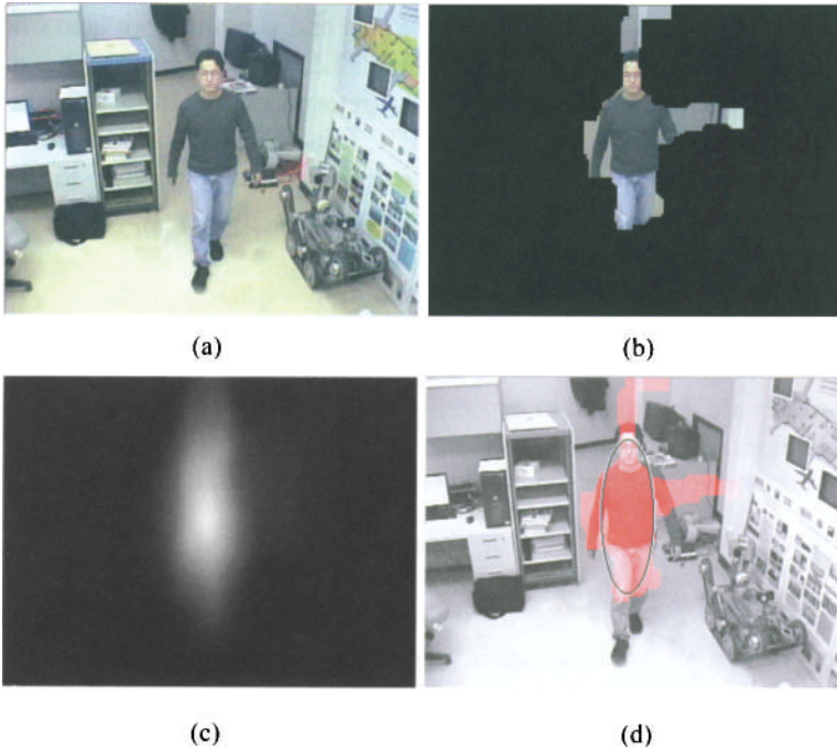
Figure 11.12. Finding a target from moving pixels. (a) One input image. (b) The extracted segment with a top-down motion. (c) The result of applying R_M = B_i * M . (d) The detected ellipse.
