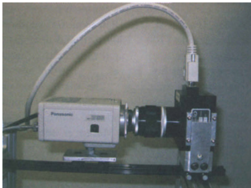
Figure 12.1. Multispectral imaging system consisting of a monochrome camera and a liquid crystal tunable filter.
