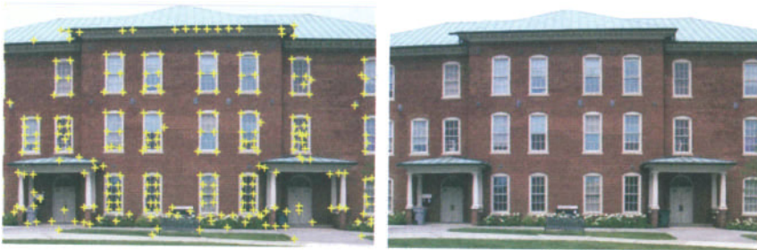
Figure 6.5. Results of Harris operator (left) applied to image "South College" (right).
