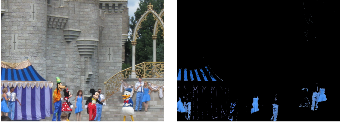
Figure 4.3: An example of image ranging: it is possible to extract the blue pants and dresses from the colourful image by choosing appropriate ranges of R, G and B values.
