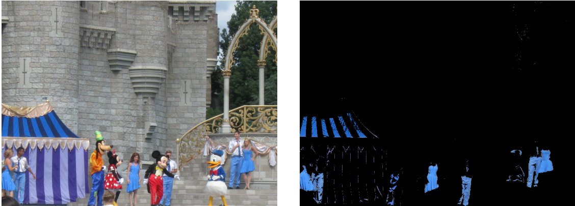
Figure 4.2: An example of image ranging: it is possible to extract the blue pants and dresses from the colourful image by choosing appropriate ranges of R, G and B values.
