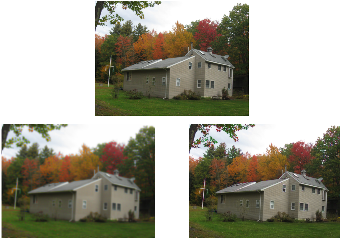
Figure 2.5: Humans are more sensitive to changes in luminance than colour. Original image (top). Effect of blurring the image luminance (bottom-left). Effect of blurring the colour information (bottom-right).
