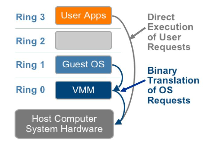
Figure Courtesy: Understanding Full Virtualization, Paravirtualization, and Hardware Assist, VMware
