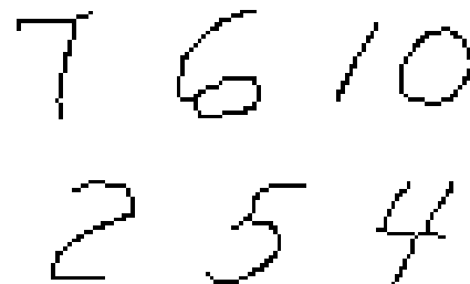
Figure 5: Skeletons of the digits in Fig. 4, thinned with the method of Zhang and Suen [28]. Note that junctions are displaced and a few short false branches occur.
