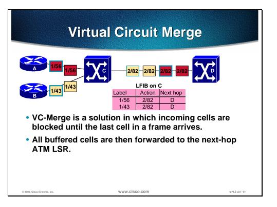
The figure illustrates the second option where the ATM switch C buffers cells coming from router B until the last cell of the packet coming from router A is forwarded.
