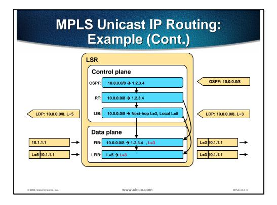
The figure shows a router where OSPF is used to exchange IP routing information and LDP is used to exchange labels.
