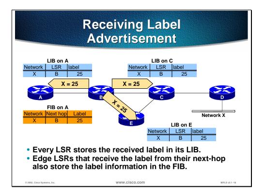
Upon receiving an LDP update, router A can fill in the missing piece in its LIB, LFIB and FIB tables:
