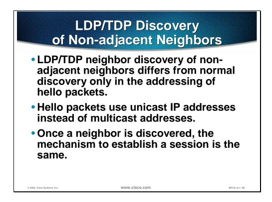
LDP can also be used between non-adjacent routers. LDP Hello messages use unicast IP addresses instead of multicast. The rest of the session negotiation is the same as for adjacent routers.
