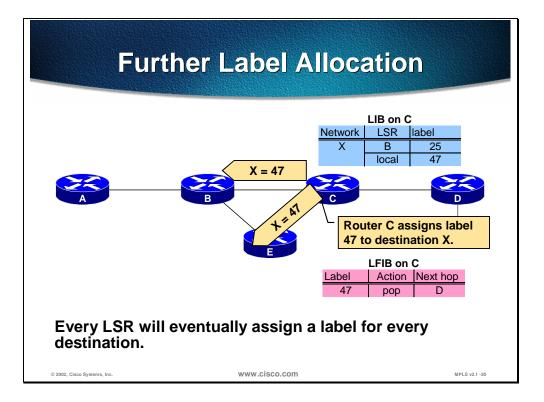
Since all routers in an MPLS domain asynchronously do the same as routers A and B, a label-switching path (LSP) is generated spanning from router A to router D.
