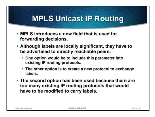
One of the applications of Multi-protocol Label Switching (MPLS) is Unicast IP routing. A label is assigned to destination IP networks and later used to label packets sent toward those destinations.
