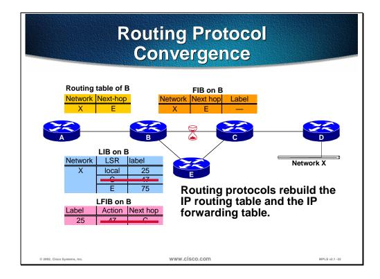
The figure illustrates how two entries are removed when the link between routers B and C fails:
