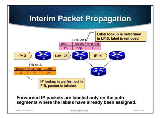
The figure shows how an unlabeled IP packet is forwarded based on the information found in the FIB table on router A. Label 25 found in the FIB table is used to label the packet.
