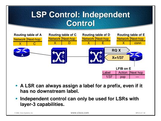
Independent control mode is usually combined with unsolicited downstream propagation of labels where labels can be created and propagated independently of any other LSR. When using independent control mode, a LSR might be faced with an incoming labeled packet where there is no corresponding outgoing label in the LFIB table. A LSR using independent control mode must therefore be able to perform full layer-3 lookups. Independent control mode can only be used on LSRs with edge LSR functionality.
