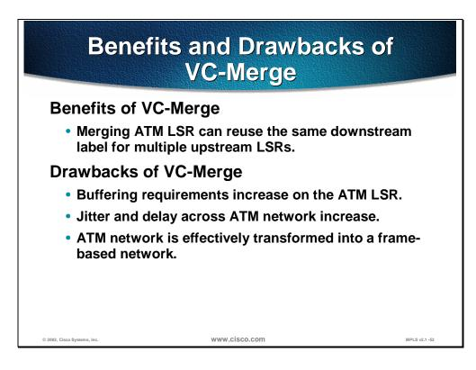
The option that buffers cells is usually referred to as "VC-Merge" because it implements the merging of two virtual circuits into one while preventing cell interleaving.
