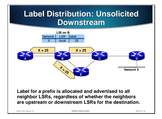
Unsolicited downstream allocation of labels is a method where each router independently assigns a label to a destination IP prefix and sends this mapping to all LDP peers. There is no control mechanism to govern the propagation of labels in an ordered fashion.
