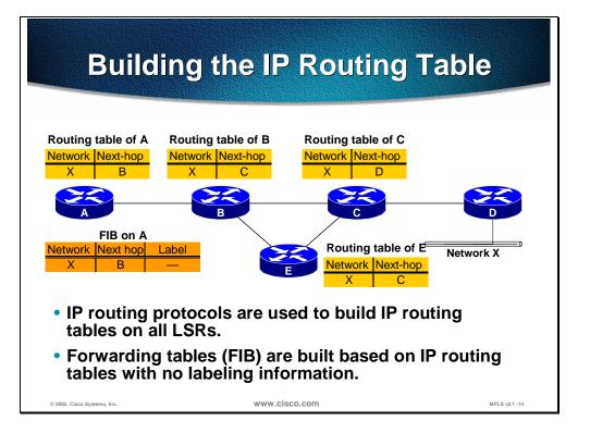
The figure illustrates how all routers learn about network X via an IGP such as OSPF, IS-IS, EIGRP, etc. The FIB table on router A contains the network X that is mapped to the IP next-hop address B. At this time a next-hop label is not available which means that all packets are forwarded in a traditional fashion (as unlabelled IP packets)
