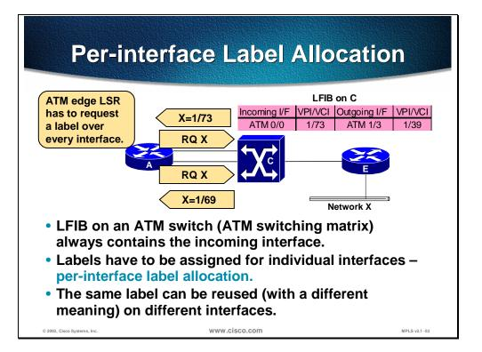
Cell-mode MPLS defaults to using per-interface label space because ATM switches support per-interface VPI/VCI values to encode labels. Therefore, if a single router has two parallel links to the same ATM switch, two LDP sessions are established and two separate labels are requested.
