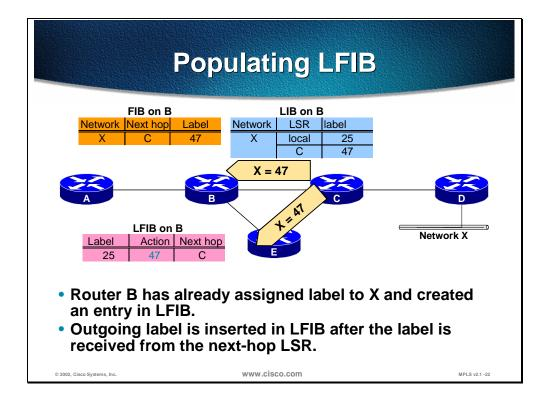
Once router C advertises label 47 to adjacent routers the label switching path (LSP) for network X has two hops:
