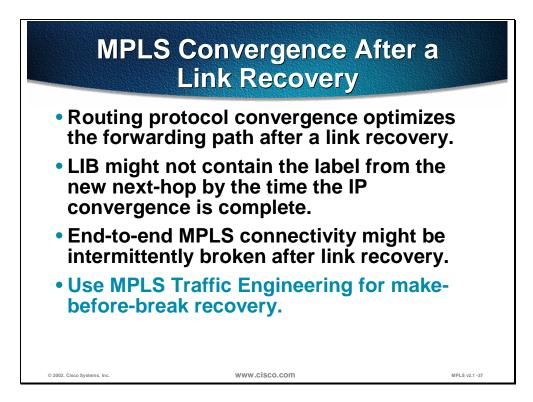
Link recovery requires that an LDP session be re-established, which adds to the convergence time of LDP. Networks may be temporarily unreachable due to the convergence limitations of routing protocols.
