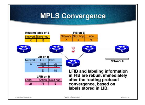
After the IGP has determined that there is another path available, a new entry is created in the FIB table. This new entry points towards router E and there is already a label available for network X via router E. This information is then used in the FIB and the LFIB table to reroute the LSP to router E.
