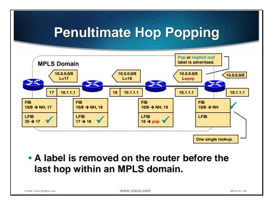
This figure illustrates how a predefined label *pop*, which corresponds to the *pop* action in LFIB, is propagated on the first hop or the last hop, depending on the perspective. The meaning of the label "pop" is to remove the top label in the MPLS label stack instead of swapping it with the next-hop label. The last router before the egress router, therefore, removes the top label.
