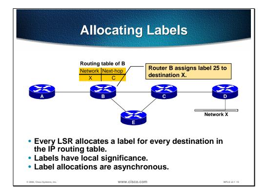
The figure shows how router B generates a locally significant and locally unique label 25 assigned to IP network X. Router B generates this label regardless of other routers (asynchronous allocation of labels).
