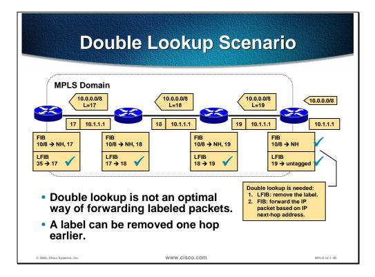
The figure illustrates how labels are propagated and used in a typical frame-mode MPLS network. The checkmarks show which tables are used on individual routers. The egress router in this example must do a lookup in the LFIB table to determine whether the label must be removed and if a further lookup in the FIB table is required.
