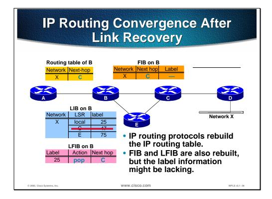
*Pop* action is used in the LFIB on router B while the LDP establishes the session between routers B and C. This process adds to the overall convergence time in an MPLS domain. The downtime for network X is not influenced by LDP convergence because normal IP forwarding is used until the new next-hop label is available.
