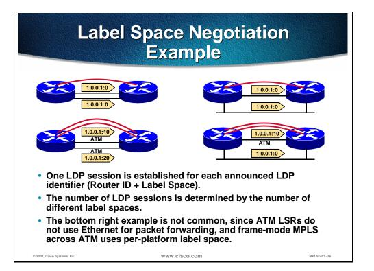
The figure illustrates four different combinations with two parallel links between a pair of routers.
