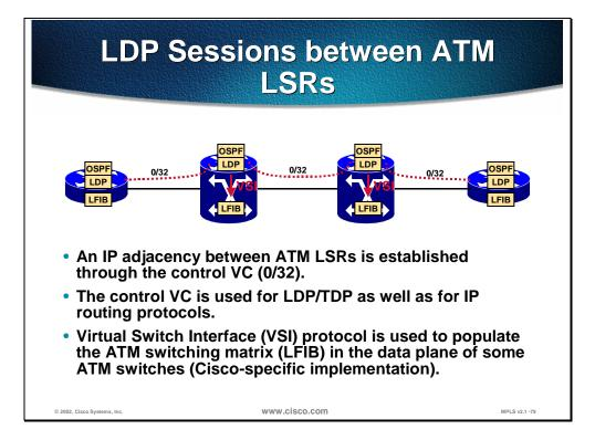
The figure illustrates the operation of LDP in ATM networks. ATM LSRs establish the IP adjacency across the MPLS control virtual circuit that by default, uses a VPI/VCI value of 0/32.
