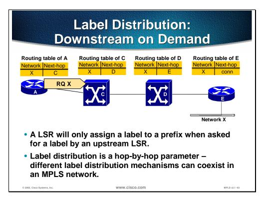
Downstream on demand allocation of labels requires each LSR to specifically request a label from its downstream neighbor. The figure shows how router A requests a next-hop label from its downstream LDP peer.
