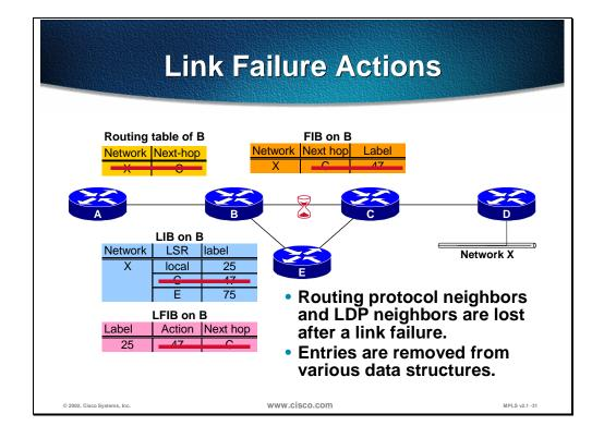
The figure illustrates how a link failure is handled in an MPLS domain:
