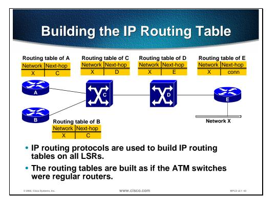
The figure shows how IP and MPLS-aware ATM switches exchange IP routing information with routers. On the control plane, each ATM switch acts as an IP router and is thus seen as an extra IP hop in the network.
