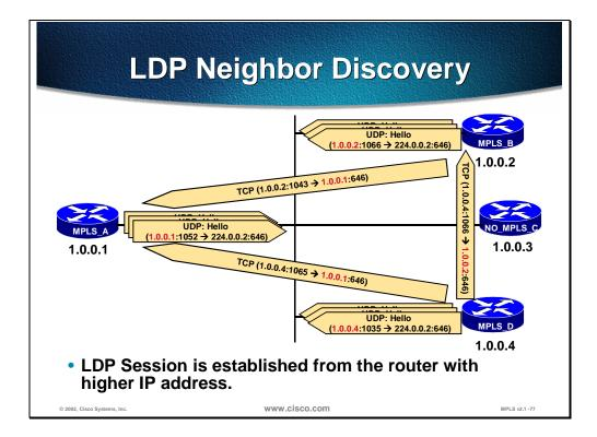
This figure illustrates how three out of four routers periodically send out LDP Hello messages (the fourth routers does not run MPLS). The routers with higher IP addresses must initiate the TCP session. After the TCP session has established they still keep sending the LDP Hello messages to potentially discover new peers or identify failures.
