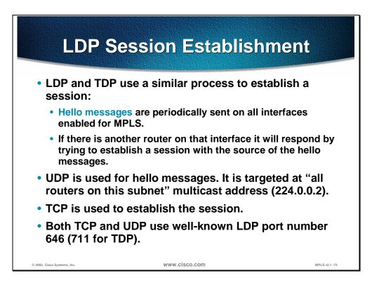
Label Distribution Protocol (LDP) is a standard protocol used to exchange labels between adjacent routers. Tag Distribution Protocol is a Cisco-proprietary protocol with the same functionality as LDP.
