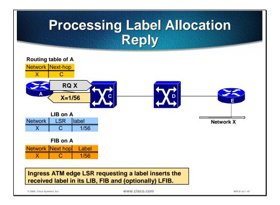
Processing of LDP replies on router A (also ATM edge LSR) is similar to the processing in frame-mode MPLS; the received label is stored in the LIB, the FIB and the LFIB tables.
