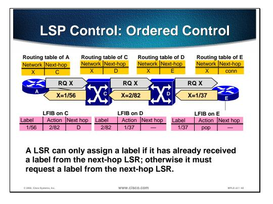
Ordered control mode is usually combined with downstream on demand propagation of labels where a local label can be assigned and propagated only if a next-hop label is available. This requirement results in an ordered sequence of downstream requests until an LSR is found that already has a next-hop label or an LSR is reached that uses independent control mode.
