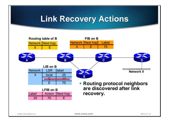
The example in the figure illustrates the actions of routers when the link between routers B and C becomes available again.
