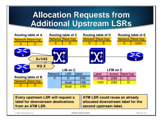
The figure shows how another router requests a label for the same destination that router A has previously requested. The ATM switch C already has a next-hop label for network X and can therefore, immediately reply to router B.
