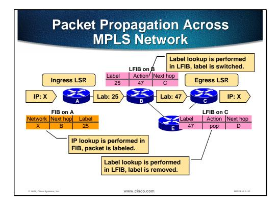
The figure illustrates how IP packets are propagated across an MPLS domain:
