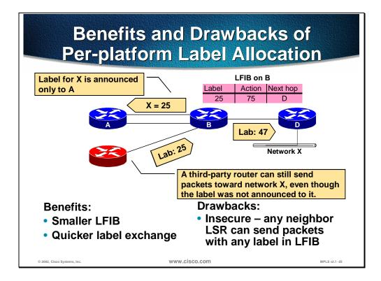
A potential drawback of per-platform label allocation is illustrated in the figure, which shows how an adjacent router can send a labeled packet with a label that has not been previously advertised to this router (label spoofing).
