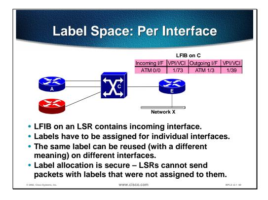
The figure shows the main difference between the LFIB table used with frame-mode MPLS and the LFIB table (ATM switching matrix) used with cell-mode MPLS.
