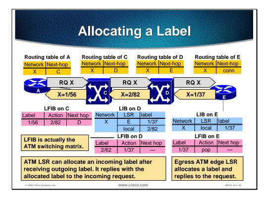
Router E replies with its local label 1/37. The ATM switch D can now generate and use its local label 2/82. Switch C receives the next-hop label from switch D and forwards its own local label 1/56 to router A.
