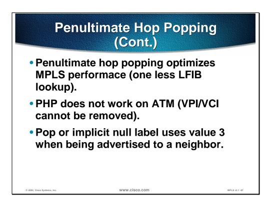
A "pop" label is encoded using a label value of 3. This label instructs upstream routers to remove the label instead of swapping it with label 3.
