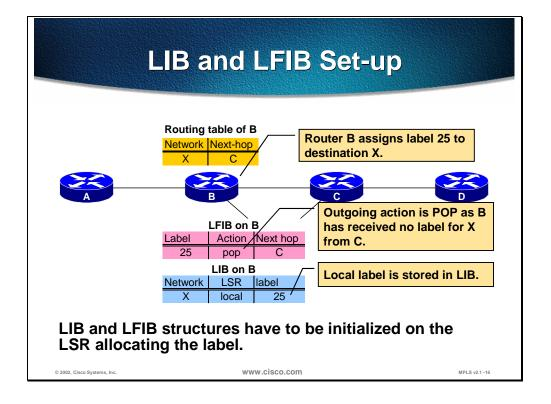
Once a label is assigned to an IP prefix, it is stored in two tables:
