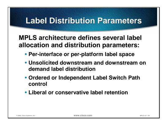
This section describes the options in label allocation, propagation and retention.
