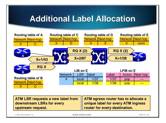
The figure illustrates the first option where an additional LSP is created for the same destination network X for every upstream ATM edge LSR. ATM switch C now has two next-hop labels for network X, one for source router A, the other for source router B.
