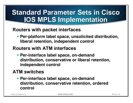
The following default operation applies to routers using frame-mode MPLS (LSRs):
