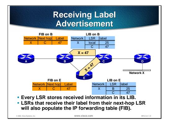
Router B can now map the entry for network X in its FIB and the local label 25 in its LFIB to the next-hop label 47 received from the downstream neighbor router C.
