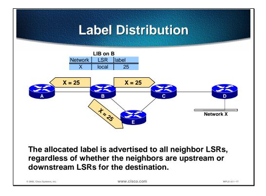
The figure illustrates the next step after a local label has been generated. Router B propagates this label to all adjacent neighbors where this label can be used as a next-hop label.
