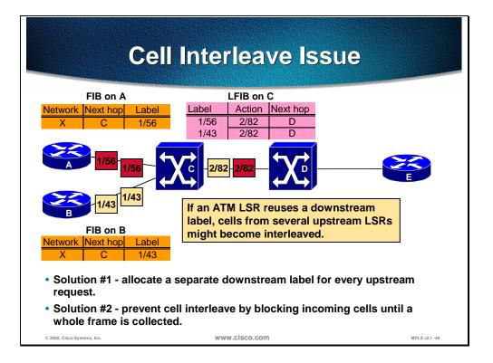
By analyzing the previous two figures it can be noted that an unusual situation has developed. Two virtual circuits from routers A and B (1/56 and 1/43) merge into one (2/82). Standard ATM virtual switching hardware does not support this and as a result segmented packets from two sources may become interleaved between the ATM switches C and D. The receiving router E is then unable to correctly reassemble those cells into two packets.
