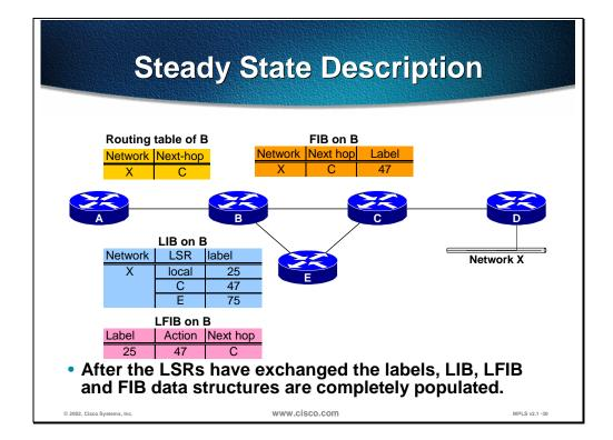
MPLS is fully functional once the IGP and LDP have populated all the tables: the main IP routing table, the LIB table, the FIB table and the LFIB table.
