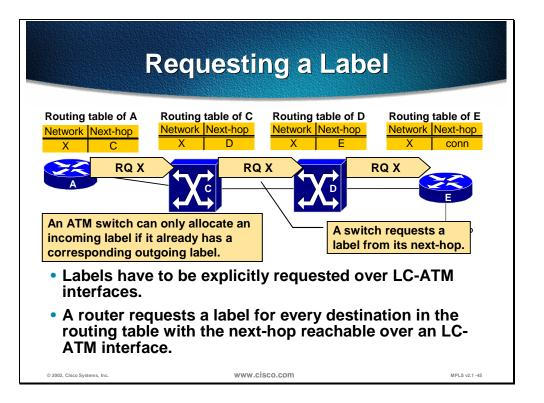
The request from router A is sent to the ATM switch C. Because the ATM switch cannot perform IP lookup, the switch is not allowed to reply with the local label unless it already has the next-hop label. If the switch does not have the next-hop label it must forward the request to the next downstream neighbor.
