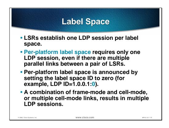
If a pair of routers is connected over two or more parallel links and use frame-mode MPLS they try to establish multiple sessions using the same LDP identifier. This results in only one session remaining.
