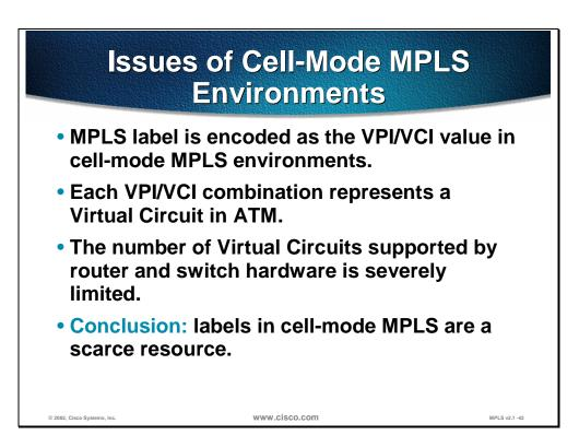
Cell-mode MPLS is significantly different from frame-mode MPLS because of some ATM specific requirements:
