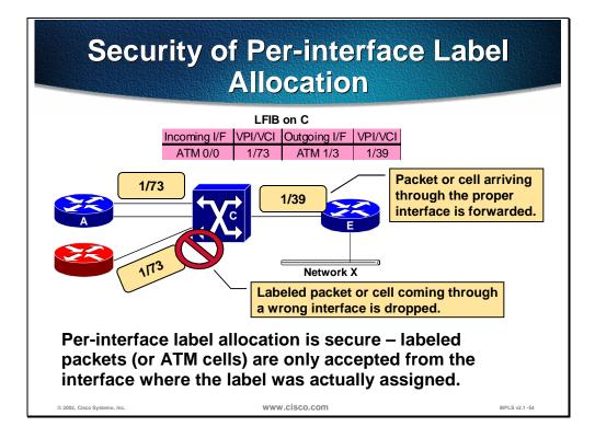
One of the benefits of per-interface label space is that it prevents label spoofing. The figure shows how the red (bottom) router tried to send a cell with a label that was advertised only to router A. The switch failed to forward the cell because it came in through the wrong interface.
