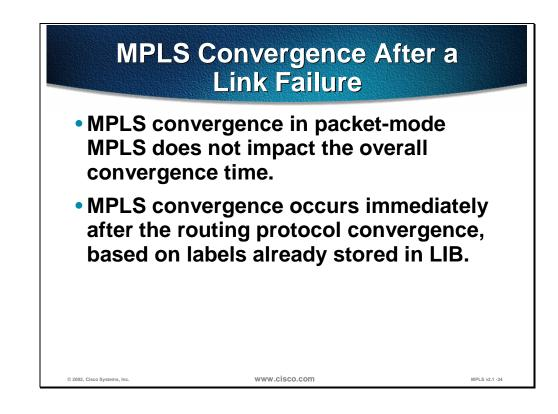
The overall convergence in an MPLS network is not impacted by the LDP convergence when a link fails. Frame-mode MPLS uses Liberal Retention Mode that enables routers to store all received labels even if they are not being used. These labels can be used after the network convergence to enable immediate establishment of an alternate label switched path (LSP).
