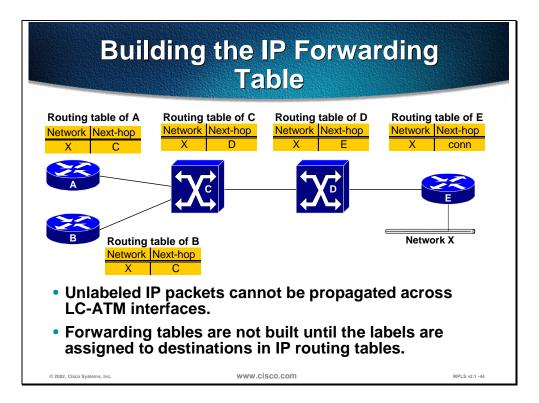
Since ATM switches are not able to forward IP packets, labels cannot be asynchronously assigned and distributed. Instead, an ordered sequence of requests is initiated by the router on the upstream side of the ATM network.
